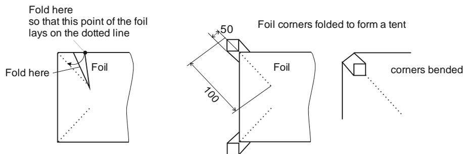
Fig. 6: Step 18: How to fold the foil
