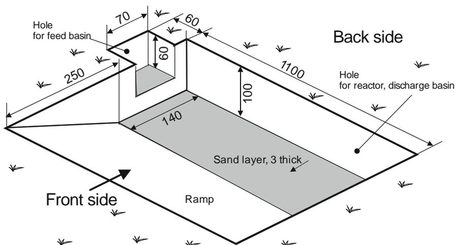
Fig. 2: Step 1–3: dimensions of the hole to be digged
