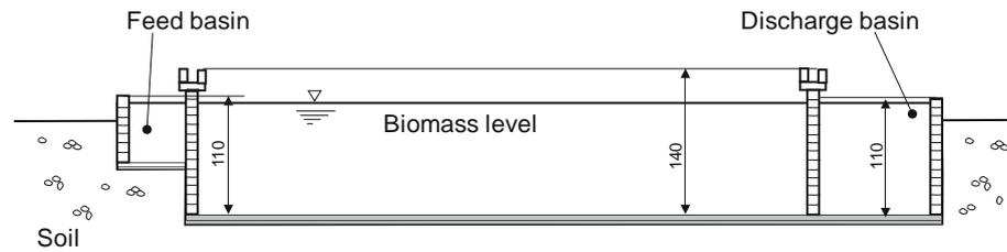
Fig 5: Cross sectional drawing of the reactor
