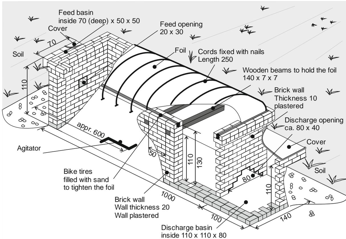
Fig. 1: Aidewise-biogas plant
